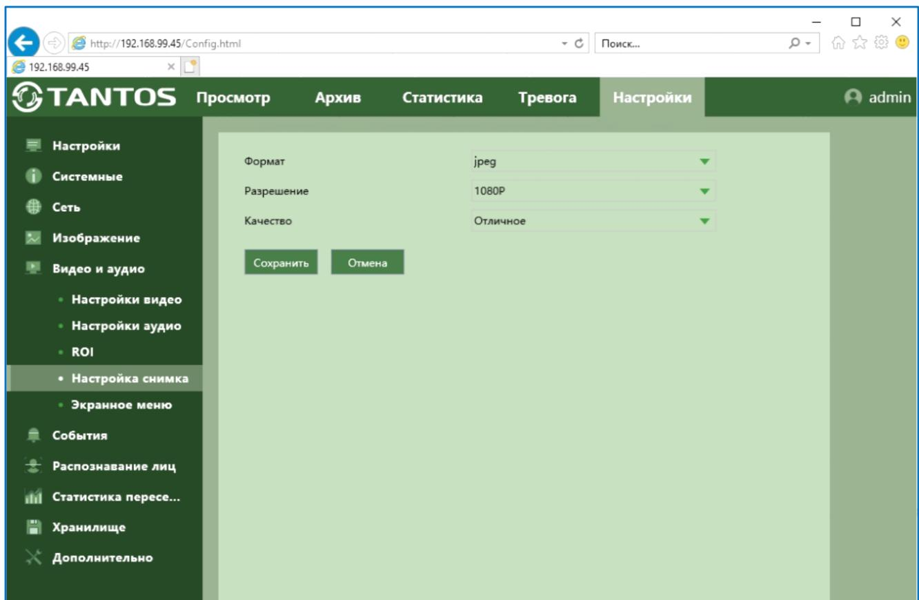
The screenshot shows the TANTOS IP camera configuration interface. The left sidebar menu is visible, with 'Настройки' (Settings) selected. The main content area is titled 'Настройка снимка' (Snapshot settings). It contains three dropdown menus: 'Формат' (Format) set to 'jpeg', 'Разрешение' (Resolution) set to '1080P', and 'Качество' (Quality) set to 'Отличное' (Excellent). At the bottom are two buttons: 'Сохранить' (Save) and 'Отмена' (Cancel).
